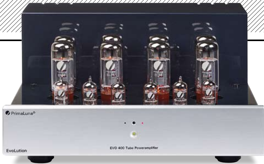
ABOVE: At 31kg, the EVO 400 power amp's bulk stems from the toroidal PSU transformer and two custom output transformers [all in screening can, behind]. Red LED on the fascia means the two pairs of EL34 pentodes (per channel) are configured in Ultralinear mode; green LED indicates triode mode
