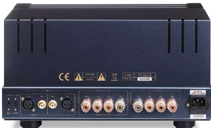
LEFT: The EVO 400 power amp has balanced (XLR) and single-ended (RCA) inputs, switched alongside. There are also three 4mm speaker outputs per channel fed from 16ohm, 8ohm and 4ohm transformer taps, respectively
