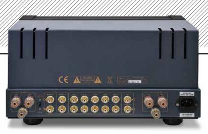
**ABOVE:** The EVO 300 offers five line inputs, an HT bypass, tape out and sub/mono line outs with a trio of 4mm speaker outputs per channel fed from 8ohm and 4ohm transformer taps, respectively. Optional MM phono module is not shown here
